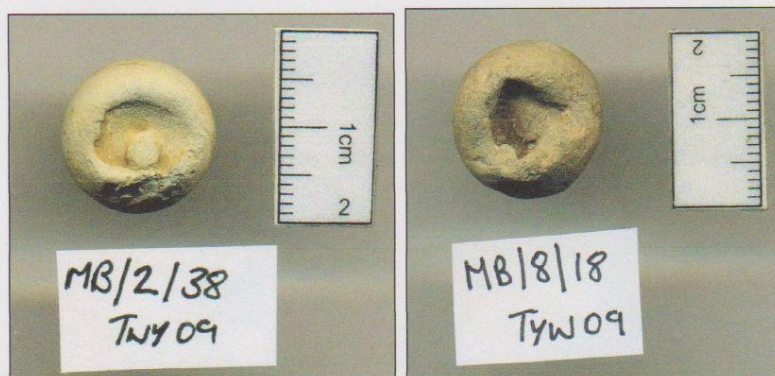
Image 2: Collapse of lead during casting
